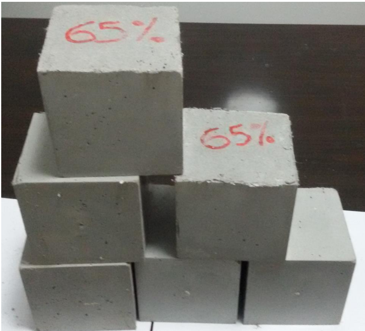
Figure 36 Photos of MSWI bottom ash concrete at 65%
