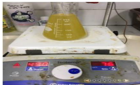
Figure 6: first stage transesterification process of methanol based biodiesel
