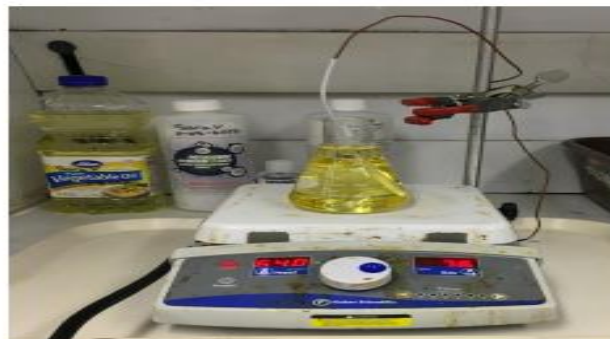
Figure 5: Heating of vegetable oil prior to the addition of alcohol
