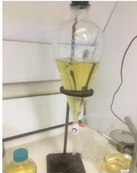
Figure 7: Second stage transesterification separation of methyl esters and glycerol
