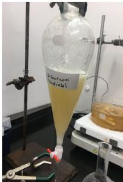
Figure 13: Saponification of 2-butanol with vegetable oil and KOH
