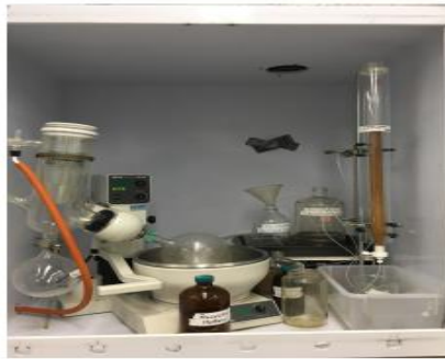
Figure 10: Biodiesel refinery apparatus used to recover excess alcohol and purify esters
