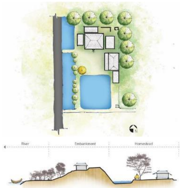
Figure (A)6.11: Layout and section of a homestead at Char Duani of Zone-A.
