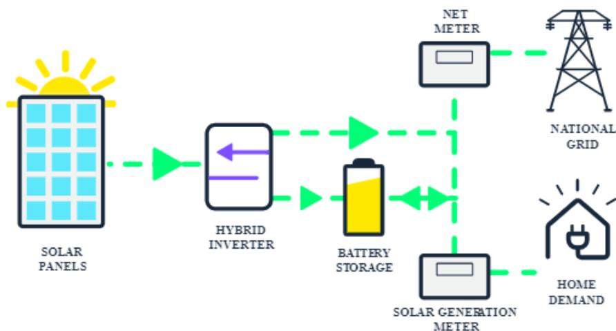
Figure 17. Hybrid Solar PV system
