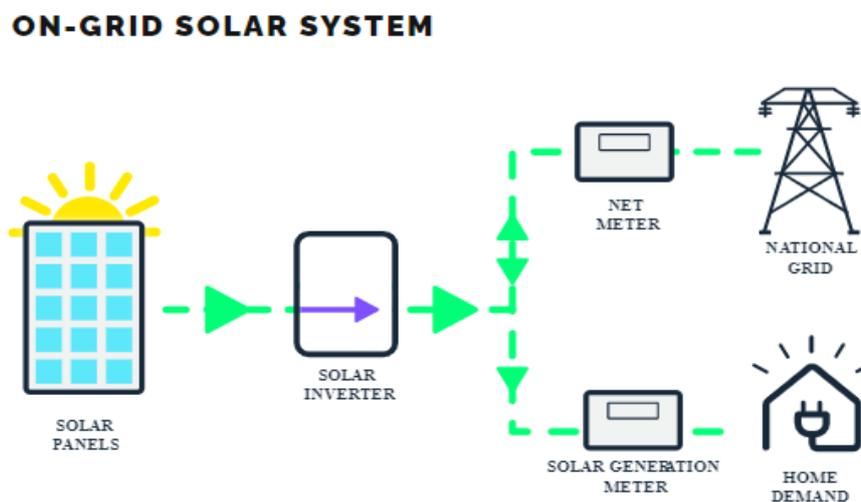
Figure 16. On-grid Solar PV system
