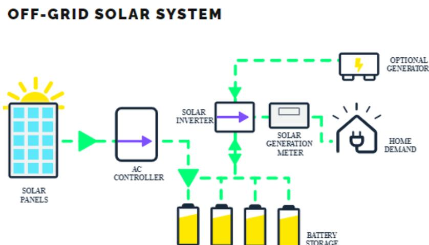
Figure 15. Off-grid Solar PV system
