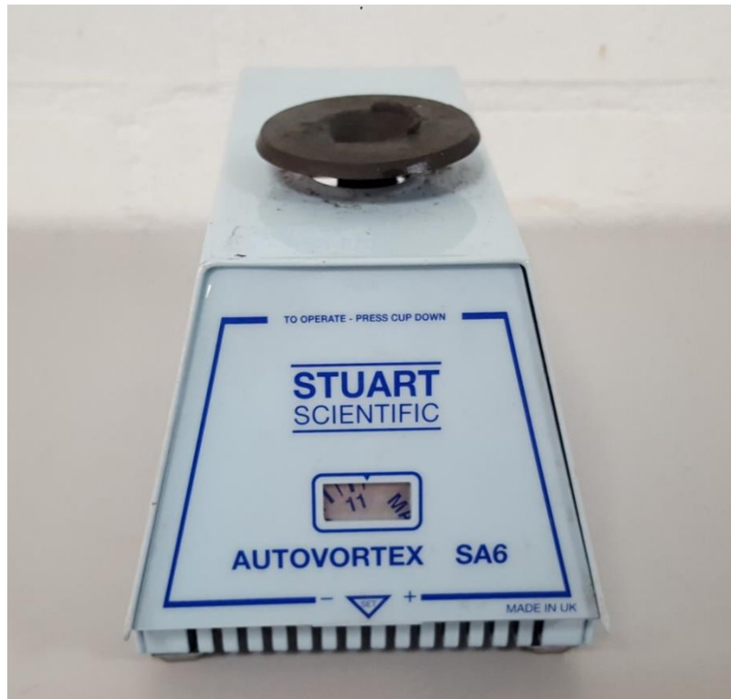
Fig. 5.15: Stuart Scientific SA6 Autovortex Vortex Mixer Lab Shaking Equipment
